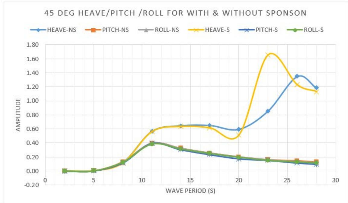
The heave motion is somehow lower (1.35m) and the peak is shifted a few seconds higher when there are no sponsons attached to the columns.
